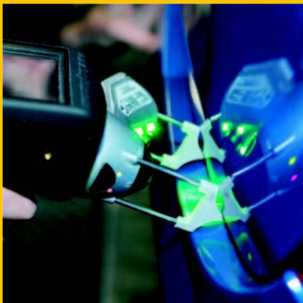
The GapGun is accurate and repeatable even in areas that are traditionally hard to measure.
